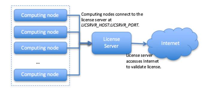
Fig. 4.1: Topology of the computing nodes and license server
